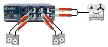
Turn the A and B outputs on or off using the front panel selectors. The LED indicators will illuminate when the output is active. Both stereo outputs can be active at the same time.
