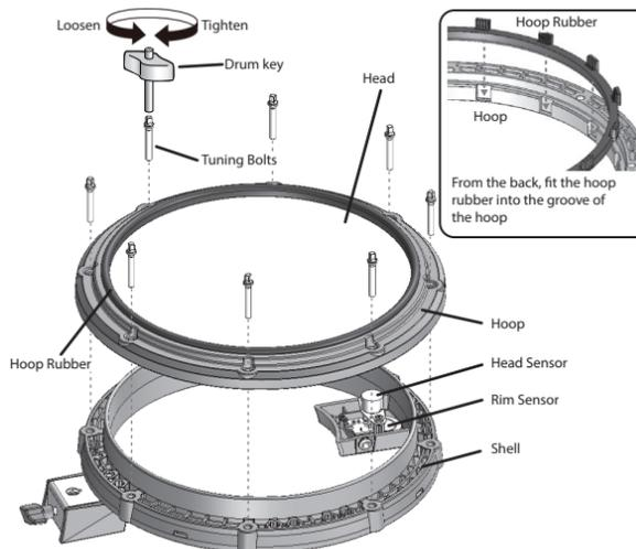
\* Do not touch the sensor section or allow foreign objects to enter it. Doing so might cause malfunction or faulty operation.
