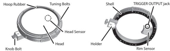
\* Do not touch the sensor section or allow foreign objects to enter it. Doing so might cause malfunction or faulty operation.
