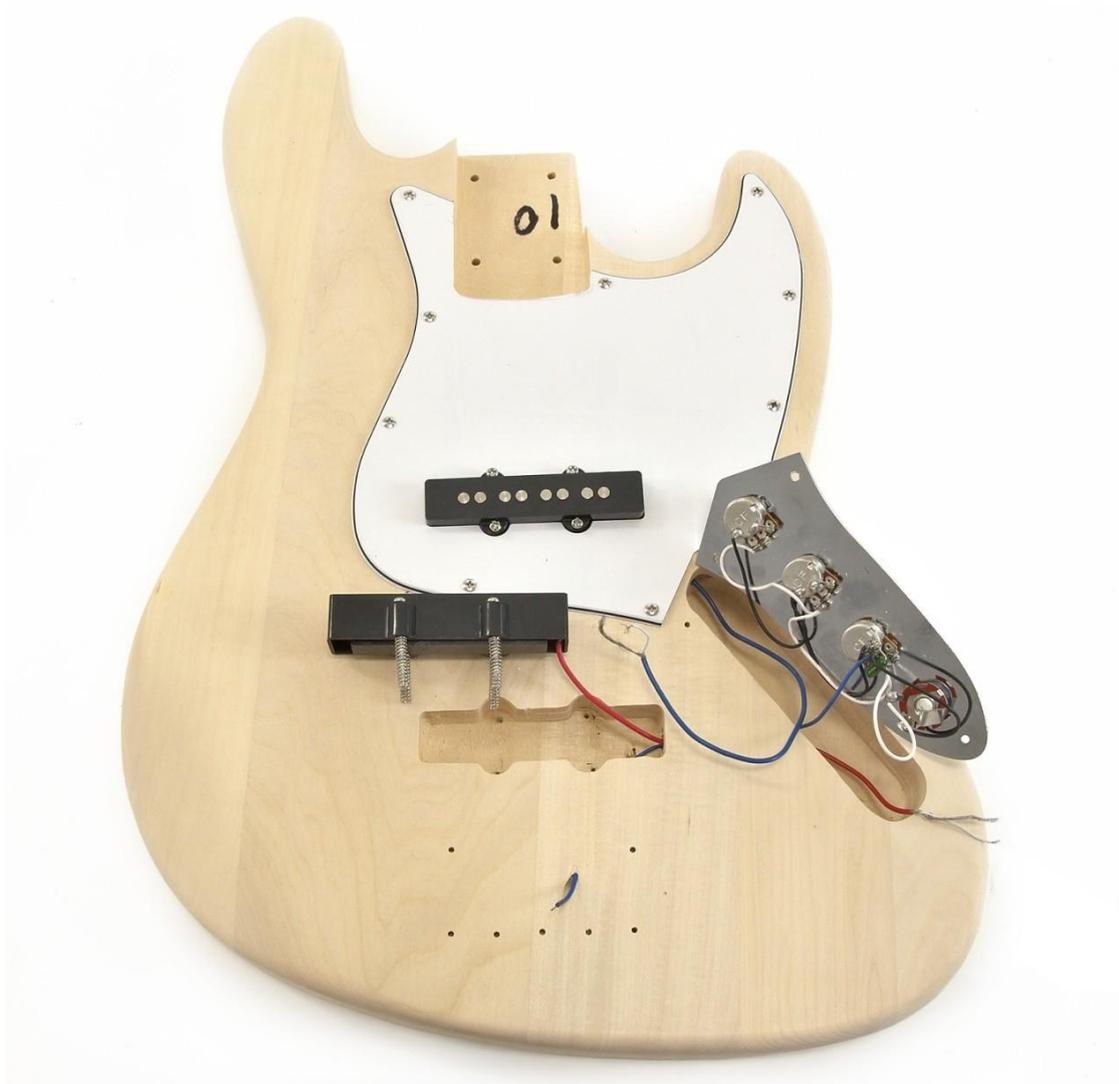
Remove the bridge pickup from the guitar body (1). Feed the blue Earth Wire (4) through the cavity in the body as shown in the picture.
