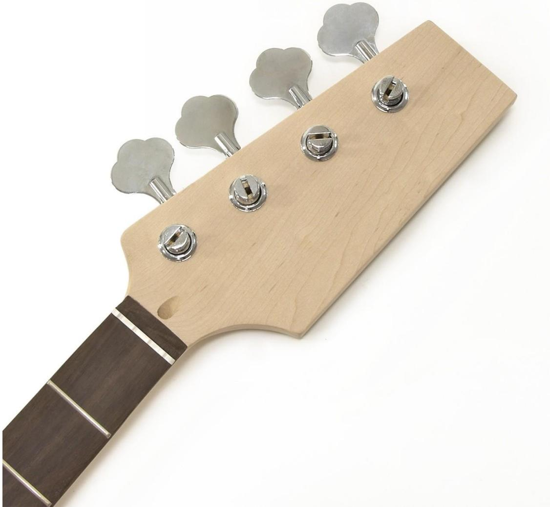
Push the Ferrules (8) into the holes on the front of the Headstock (2). Turn the neck over and screw the machine heads (7) in place using the 16x7mm (thin) screws.
