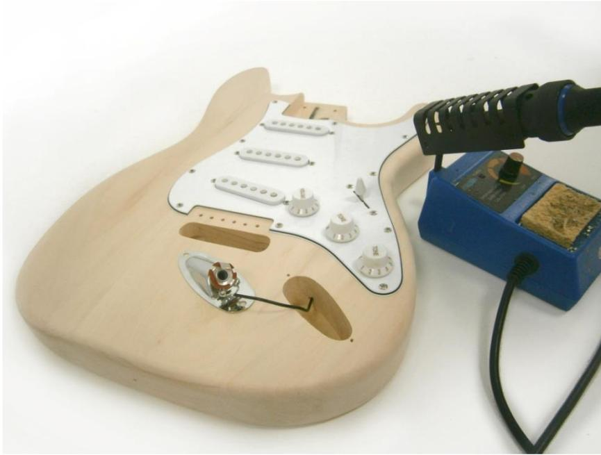
Attach the Jack Plate (4) to the wires on the front of the body (1) using the solder provided (15). The white wire should connect to the top arm of the jack input, and the red wire to the bottom arm. The Jack Plate (4) should then be placed to match the pilot holes on the front of the body using two of the 6mm screws.
