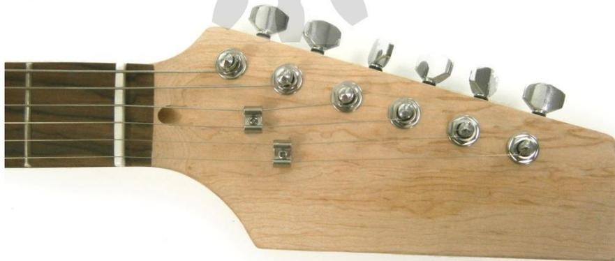
String the guitar and then attach the String Trees (13) to the Headstock (2) using the 7mm and 8mm screws and the small spacers. The 8mm screw and larger spacer should be placed between the D and G strings, and the smaller spacer and 7mm between the B and E strings.
