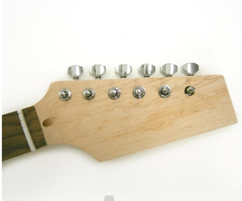
Insert the machine heads (3) in to the holes in the Headstock (2). Place the washer (12) on top, and then screw in the Ferrules (11). The neck should then be turned over and six of the 7mm screws should be screwed into the pilot holes securing the machine heads in place.
