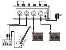
Can use the dual output channel connection of multi-effects, or MOOFR Micro ABY MK II
