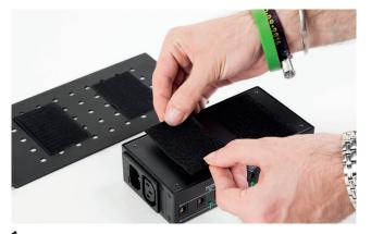
**1.** Take the RockBoard<sup>®</sup> The Tray and fix your power supply to it. We recommend the use of hook & loop tape or cable ties.
