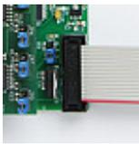
House the FH-1 in a Eurorack case of your choosing. The power connector is [Doepfer standard](#). If using the power cable supplied with the FH-1, the red edge of the cable is nearest the bottom of the PCB, and carries -12V. ("-12V" is marked on the PCB itself next to this end of the connector.) Be sure to connect the other end of the power cable correctly, again so -12V corresponds to the red stripe on the cable.
