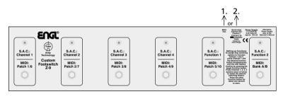
**2. ENGL Custom Z-9 Footswitch:** This special foot board connects to the preamp via a <sup>1</sup>/<sub>4</sub>" stereo cord plugged into the Serial Amp Port (58) or via a 5-pin DIN cord plugged into the MIDI IN port (55). The former option affords switching access to channels and two special functions (for example, *Hi Gain* or *Mega Lo Punch*). In the latter setup, the Z-9 serves as a MIDI foot board that accesses the first 10 MIDI presets.
