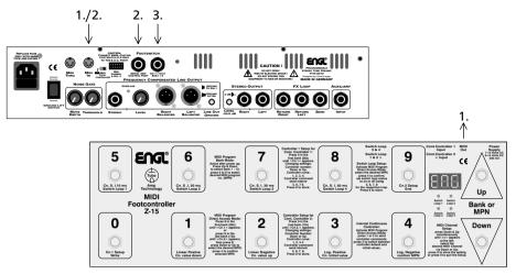
**1. MIDI foot board (for example, the ENGL Z-12 or ENGL Z-15 pictured above):** Connect the foot board to the preamp using a standard 5-pin DIN cable. All 5 terminals of both connectors must be wired in a 1:1 configuration: MIDI data transmission requires two wires, and the ENGL MIDI foot board uses two more wires for purposes of power supply. This combination affords access to all of the amp's 128 MIDI presets. The Z-15 foot board also lets you control Master Volume Mute via MIDI controller.
