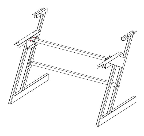
2. Connect the main shelf cross bracket to the main legs, attach the keyboard shelf and tighten the screws.
