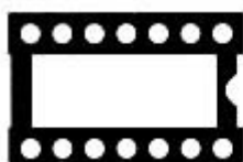
IC-socket with marker notch
