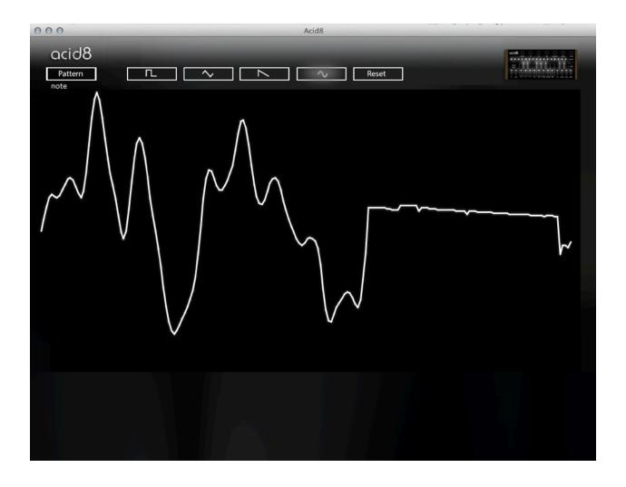
Now you can visualize and redraw the **4th waveform** of each shape in real time with your mouse. These changes are automatically saved to ACID8s memory. Use the reset button to restore the factory waveform.
