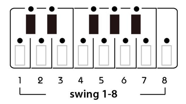
Hold shift, then press **swing** (white key #7) to enter swing mode. While keeping shift held you can now select the level of swing by pressing any of the white keys.
