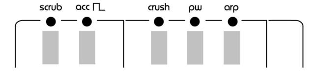
To toggle an effect on or off, hold shift whilst pressing any of the black keys
