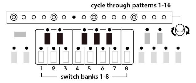
Roll the encoder to cycle through the 16 patterns of a bank. Switch banks by pressing any of the white keys.
