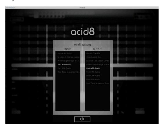
Note: INPUT is the port receiving data **from** Acid8. OUTPUT is the port **to** Acid8.
