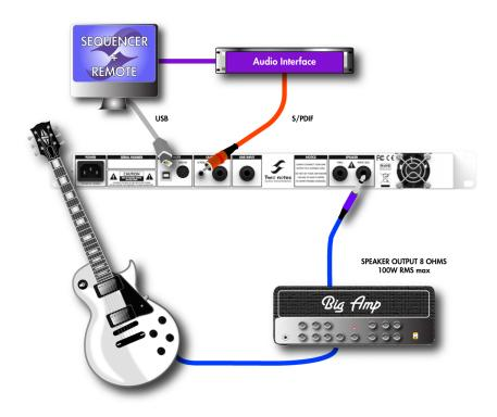
Plug your 8 ohms out on your amplifier to the SPEAKER input of the TORPEDO *Live*. If you want to use a preamplifier, plug its line output to the LINE INPUT of the machine.
