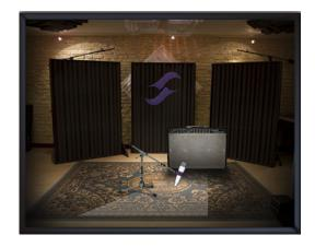
In the "MIKING" menu, you take the place of the sound engineer. This is where you will find the "sweet spot", the perfect microphone position. You will also be able to control speaker saturation and balance between simulated and non-simulated tones. The first two parameters determine the microphone's position. You can move the microphone around inside a trapezoidal plane that the **Torpedo Remote** software lets you visualize.
