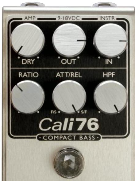
**Percussive, lively & fat.** A slow attack time allows the compressor to accentuate the initial transient of any given note. Fast release allows the compressor to fully recover between notes, so that every phrase and chord will take on a percussive quality. Low ratio keeps compression artefacts / distortion to a minimum. High HPF results in fattened low bass frequencies.
