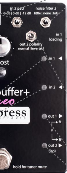
**noise filter:** helps eliminate certain types of noise from your signal path, especially white noise and hiss generated from digital pedals. It will reduce this noise on any pedal that is inside its dedicated loop.
