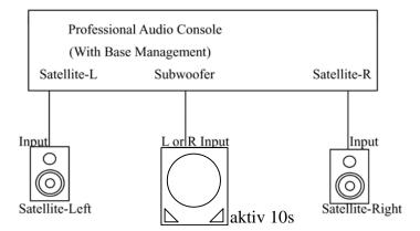
In a 5.1 or a 7.1 setup, the other surround speakers will also be connected to the source directly although the diagram does not show that. If your source device is only stereo and / or does not have its own base management, the satellites are connected to the outputs on the right side of the back panel of aktiv 10s using balanced XLR cables. Refer to the following diagram:
