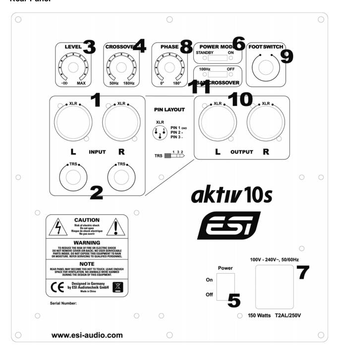
**1. XLR inputs** – these connectors accept balanced XLR input connections. The XLR input is wired like this:
