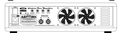
**LINE INPUT** - The rear panel has a Line Input socket for connection of other signal sources into the system. This can be used for plugging a CD, Tape or MP3 player into the amplifier for practising, rehearsing or for connection of a second pre-amp into the system.
