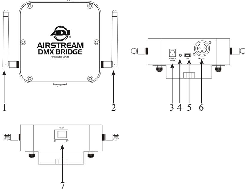
1. **Wi-Fi Antenna** – signal between bridge and Wi-Fi device.
