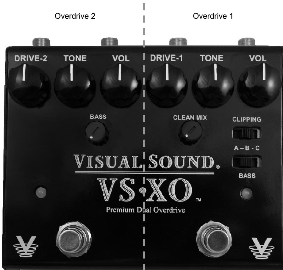
Overdrive 1: Typical Drive, Tone (high boost / cut), and Volume knobs, plus...
