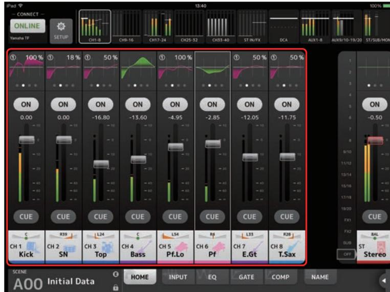
Channel strips for 8 channels are displayed in the details area. You can scroll left and right to display the channel strips for other channels by swiping left or right on an inactive area of the screen.
