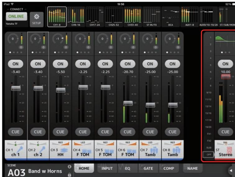
The STEREO channel strip is normally displayed in the overview strip area. When using SENDS ON FADER mode, the destination AUX channel or SUB channel strip is displayed here.
